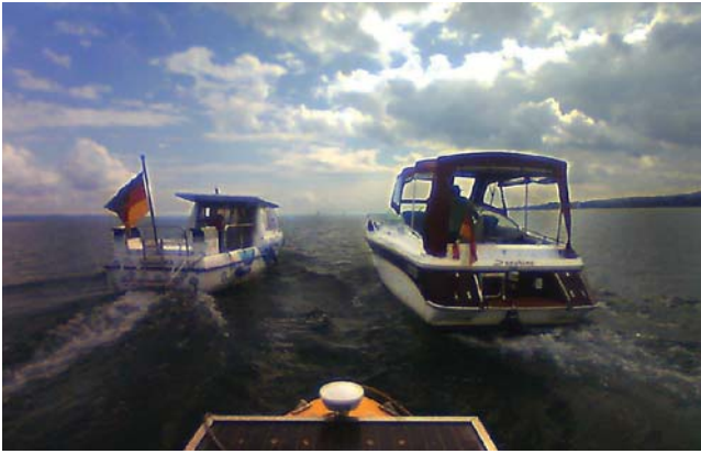
Fig. 10. Target vessels used for data acquisition. The left one (blue) is also used for the single object scenario and has a size of 8.5 \text{ m} \times 2.5 \text{ m} . The dimensions of the right one (red) are 6.9 \text{ m} \times 2.47 \text{ m} .
